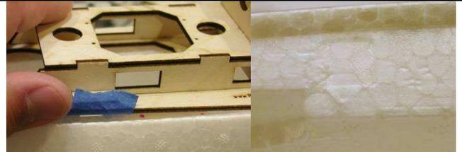
11. Cut out the foam to allow the magnets to sit recessed in the fuselage. Leave enough area for the epoxy to fill in.
