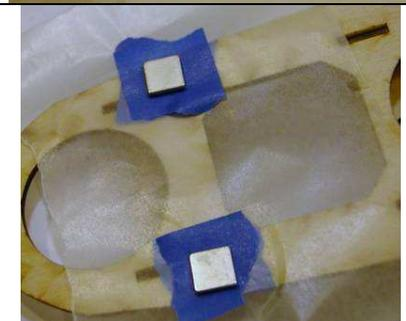
13. Fill the cutouts in the fuselage with 5 minute epoxy, leaving enough room for the magnets to be inserted.
