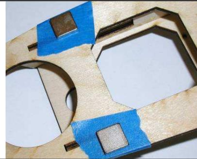
10. Place the pod into the cockpit area and press the magnets into the foam to leave indentations.
