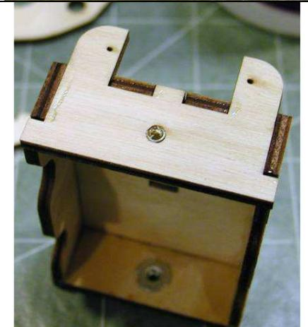
Attach the rubber-band catch as shown.
