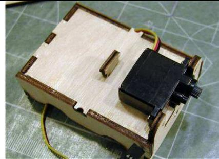
Attach the side pieces to the base plate as shown (note orientation of sides and location of center hole).
