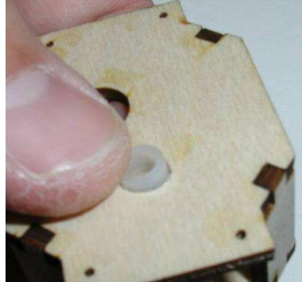
Install small washer and aluminum spacer on the bolt as shown.
