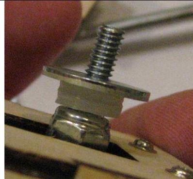
Place tilt platform on bolt. Place tooth-lock washer and nut on until it just starts to snug down (standard tilt module shown, GoPro tilt mounts using the same method in the center hole on the base).
