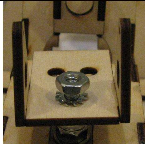
Center the servo and place tilt platform pointed 180 degrees from the desired direction. Hold the bolt with a screwdriver (DO NOT APPLY FORCE AGAINST THE SERVO). Rotate the tilt platform, making sure the bolt is moving, until the bolt is tight and the platform is facing the proper direction.
