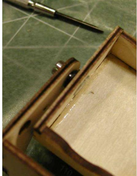
On the opposite side, insert the shoulder screw as shown and add the two washers. Pull the shoulder screw back so it just barely holds the two washers and move the camera holder in place. Tighten the shoulder screw into the tee nut.
