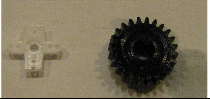
Apply a thin layer of epoxy to the top of the servo arms and place it on the gear. Make sure the arm is centered in the gear (look through the opposite side to make sure the holes line up). Be careful to not get any epoxy on the gears. Quickly wipe excess epoxy away using alcohol on a rag if needed.
