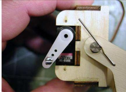
Slight control rod into the EZ Connector and tighten securely when camera is pointed directly forward when the servo is centered.
