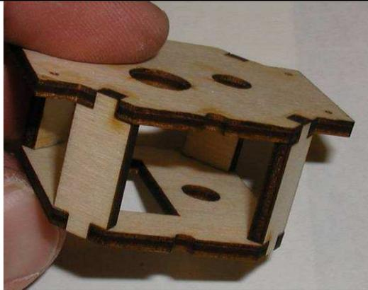
Verify aluminum spacers slides smoothly through holes on top and bottom plate. If force is required, scrape the hole with an X-Acto knife until the spacer slides through easily.
