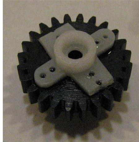
Insert the gear in the large hole and insert servo into gear. Tighten screw to retain servo horn through the hole in the gear center.
