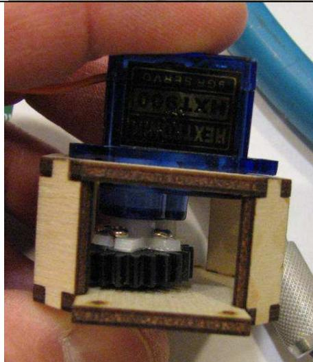
Verify that the gear is aligned and the servo is seated properly. Drill pilot holes for the servo screws and hold servo in place with screws.
