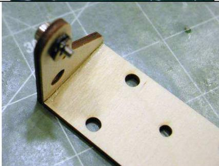
Screw the shoulder screw into the tee nut as shown.
