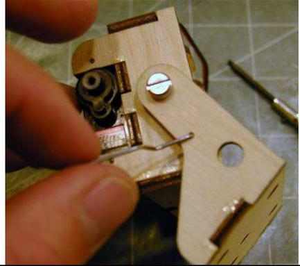
Place servo horn on servo so that the angle is approximately the same as in the picture when the servo is centered.
