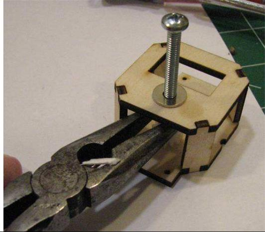
Install aluminum spacer and second small washer as shown
