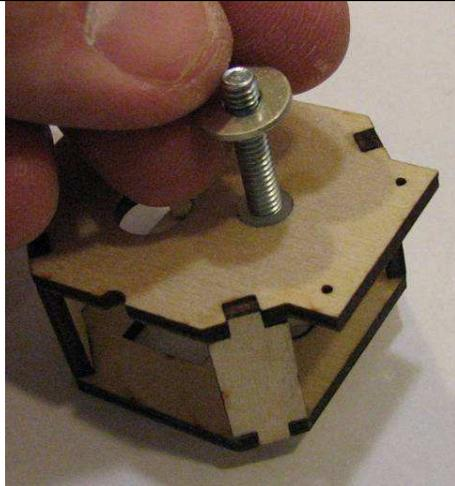
Install the lock nut until snug. Verify free movement of assembly. If gear assembly does not move freely you may back off the lock nut slightly. If it still does not move freely, disassemble the components and verify the spacers fit loosely in the holes. If needed, scrape the inside of the holes with an X-Acto knife until the spacers slide freely through the holes.
