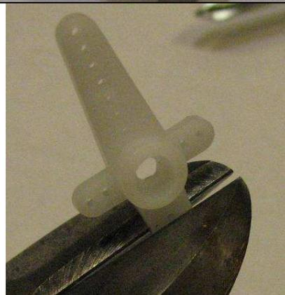
Sand the top surface of the servo arm and the side of the large gear to roughen.
